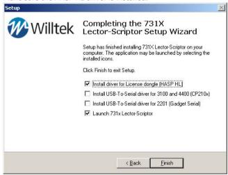
4 When the installation is completed, start Lector (if it does not start automatically). Define the connection between the PC and your instrument by selecting **Connection > Define Interface**.
