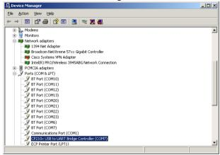
Look for the CP210x USB to UART Bridge Controller connection and check which COM port it uses.
