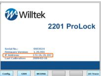
If the ProLock displays an IP address of 0.0.0.0, it is not properly connected to the LAN or the computer. Check the configuration of the 2201 ProLock, the Ethernet settings and the cable connections.
