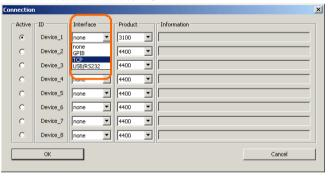
Check the IP address which is displayed in the acknowledge messge displayed after connecting via USB or RS-232 (see step a on page 21 and step b on page 22).
