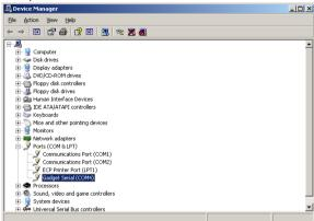
Apply the COM port number in the Connection menu within Lector. The baud rate should be set to 115200.
